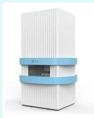
Nanoparticles that reach and bind to the target cells (Néel relaxation) are measurable by superconducting quantum interference device (SQUID) magnetometers (MRX instrument developed in house), while unbound nanoparticles (Brownian motion) such as those freely circulating in the bloodstream are not detected and bone and normal tissue do not produce any magnetic signal.
